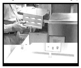
5) Using a wire grill brush or dry abrasive pad, clean exposed surface of Conveyor Belt by passing brush or pad, back and forth across the surface of the Conveyor Belt.
