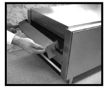
2) Remove Tunnel Extender by first removing screws as shown and lifting up and away from oven.
