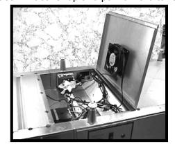
4) Using a vacuum, clean fan motor and inside of control box.
