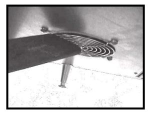
5) Return unit to counter and remove screw holding power supply side panel in place. Carefully lift panel up and out. Two ground straps hold panel to oven chassis. **DO NOT REMOVE GROUND STRAPS**OR DISCONNECT POWER SUPPLY CORD. Vacuum any dust and debris from inside of unit (repeat for opposite side).
