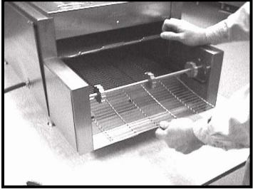
(NOTE: TO PREVENT DAMAGE TO ELEMENTS, DO NOT LET GO OF CONVEYOR BELT.)
