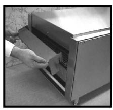
4) Remove Tunnel Extender by first removing screws as shown, and lifting up and away from unit.
