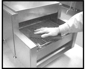
6) When section of Conveyor belt is clean, remove wire brush or abrasive pad from conveyor surface. Reconnect power or turn power back on. Turn the ON/OFF switch to the **ON** position. Allow the Conveyor Belt to advance to expose another section of belt surface. Turn the ON/OFF switch to the **OFF** position. **Disconnect or turn power off at wall breaker**.
