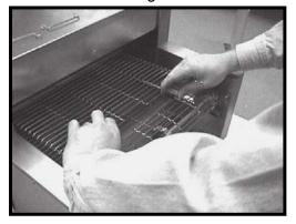
14) Working from either side of Conveyor Belt, use Master Clips to connect both ends of Conveyor Belt as shown below.
