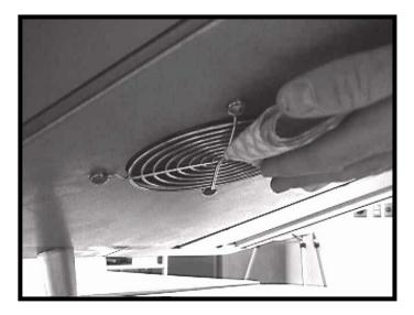
6) Check beneath oven to make sure there are no obstructions to the air intake as shown below.
