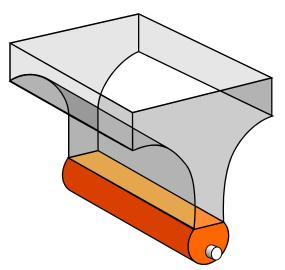
Bottom-fired fryer with a cool zone limited in size by the shape of the tank design and burner placement continuous bottom firing causes heat to conduct to tank bottom thus causing loss of cool zone.
