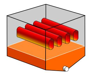
Pitco's cool zone is larger; the tube fired design creates a substantially larger cool zone for trapping particles thus prolonging oil life and reducing taste transfer
