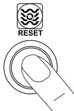
**NOTE:** If the burner does not light within 15 minutes, the oven enters a safety lockout mode that disables the "RE-SET" switch. If this occurs, turn the "HEAT", "BLOWER", and "CONVEYOR" switches to the "OFF" ("O") position. Wait for AT LEAST FIVE MINUTES. Then, repeat the Daily Startup procedure.
